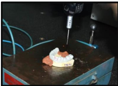
Fig. 1: Measurement using a 3-dimensional Coordinate Measuring Machine
