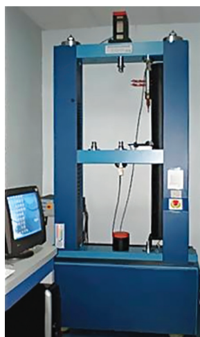
Fig. 2: Specimens being loaded in the universal testing machine
